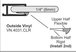
Used on vertical wall channels, angled posts and sills
