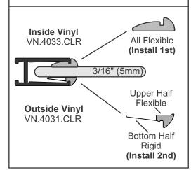
Used on vertical wall channels, angled posts and sills
