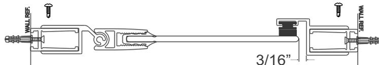
3 Before installing the full length magnet, clean the door glass. Please note the polarity of the magnet in the latch jamb and magnet with the adhesive. Apply the magnet to the glass by peeling off the backing and applying it down the edge of the glass as shown. Adjust the strike to work correctly with the magnet in the rail and to be plumb. If the magnets repel each other, reverse the magnet strip in the latch jamb. Secure the top, middle and bottom of the strike with #8x1/2" tek screws.
