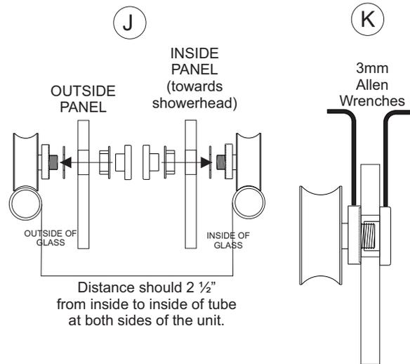
**STEP 11 - Install Center Guide:****\* Move both panels middle of header tubes.****\* Slide the Center Guide under both panels and align with marks made in STEP 3.**
