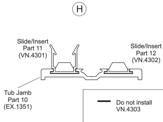
**STEP 13 - Cut and Install Tub Jambs:** reference diagram below
