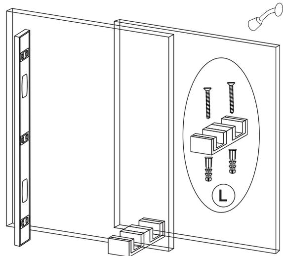
**STEP 12 - Prepare Tub Jamb:****\* Insert one piece of vinyl (11) and into the "T" slot****\* Insert one piece of vinyl (12) into the other slot. Orient the vinyls as shown.****\* Repeat for second Tub Jamb****\* Do not install vinyl (13). You will do this after the jambs are screwed to the walls to cover the screw heads.**
