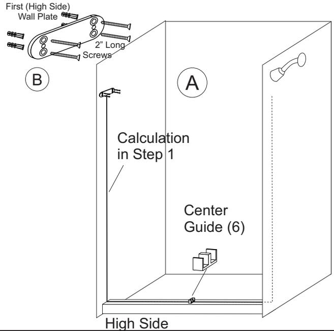
**STEP 4 - Mount First Wall Plate on High Side:**
